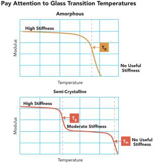
The graphs show typical changes in modulus for amorphous and semi-crystalline plastics as temperature changes. Glass transition temperatures typically are not included in standard data sheets used by design engineers.
