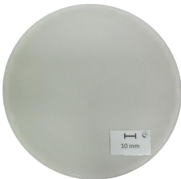
Macrosection, d178 mm: segregation zone 3.1 mm
